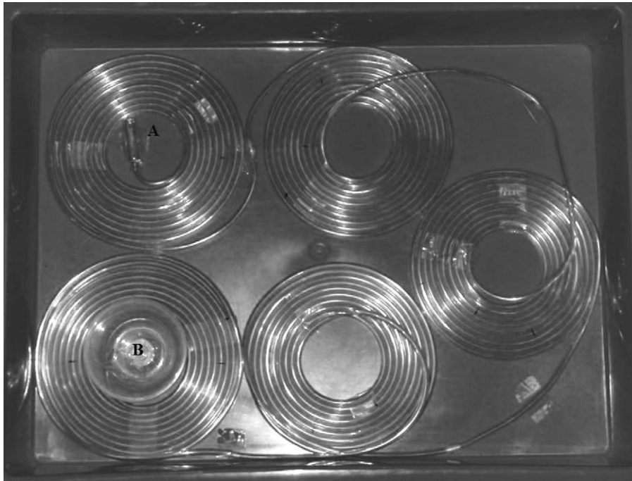
Fig. 1. The modified extended arena for studying C. hemipterus active movement activity: (A) point of introduction (glass vial) and (B) point of termination (plastic container).
